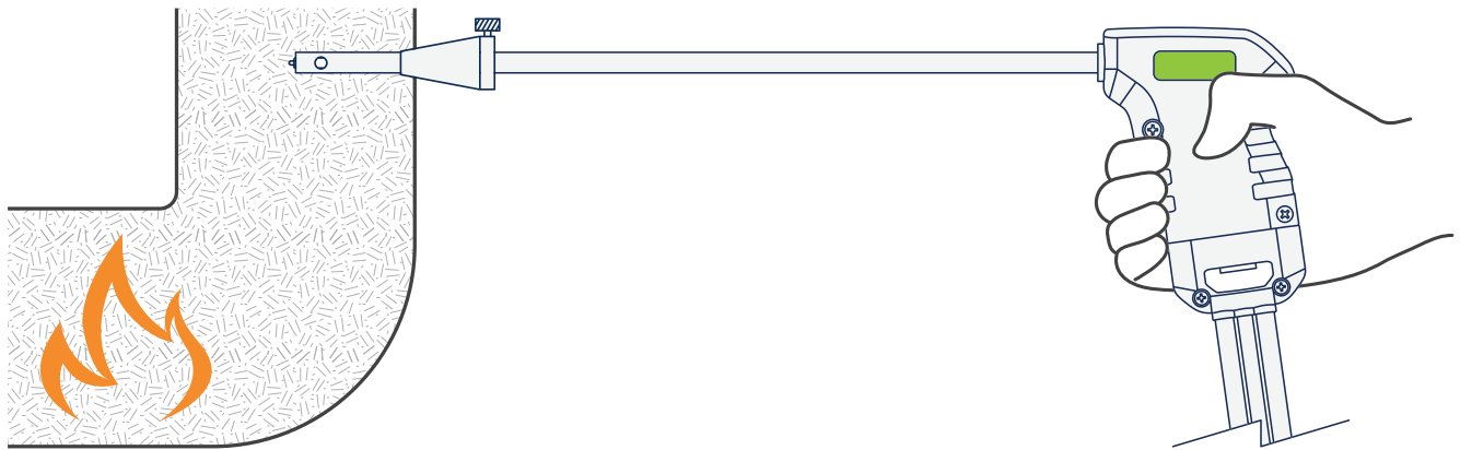
Fig. 3-6: Probe Placed in Center of Measurement Area
